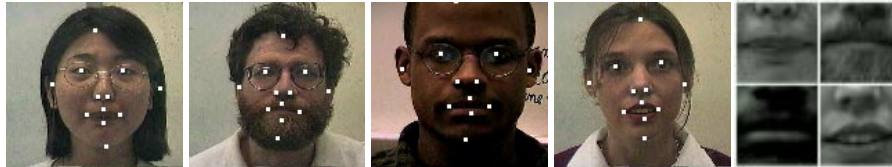
Figure 2: Sample frames from four database subjects, with detected facial features superimposed ( left ), and grey-scale, 64 \times 64 pixel, mouth regions of interest extracted ( right ).
