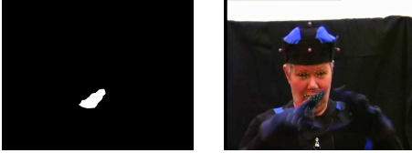
Figure 3. Example ground-truth data: The left image shows the binary mask for the image displayed on the right. White pixels in the mask denote the occluded pixels. The ground-truth landmarks are overlaid on the image on the right.
