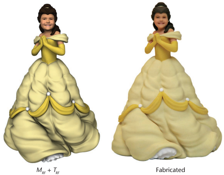
Figure 10. The system fabricates the completed customized CG figurine ( M_{RF} ) with a customized texture map ( T_{RF} ), using a color 3D printer. We use a ProJet 660Pro.
