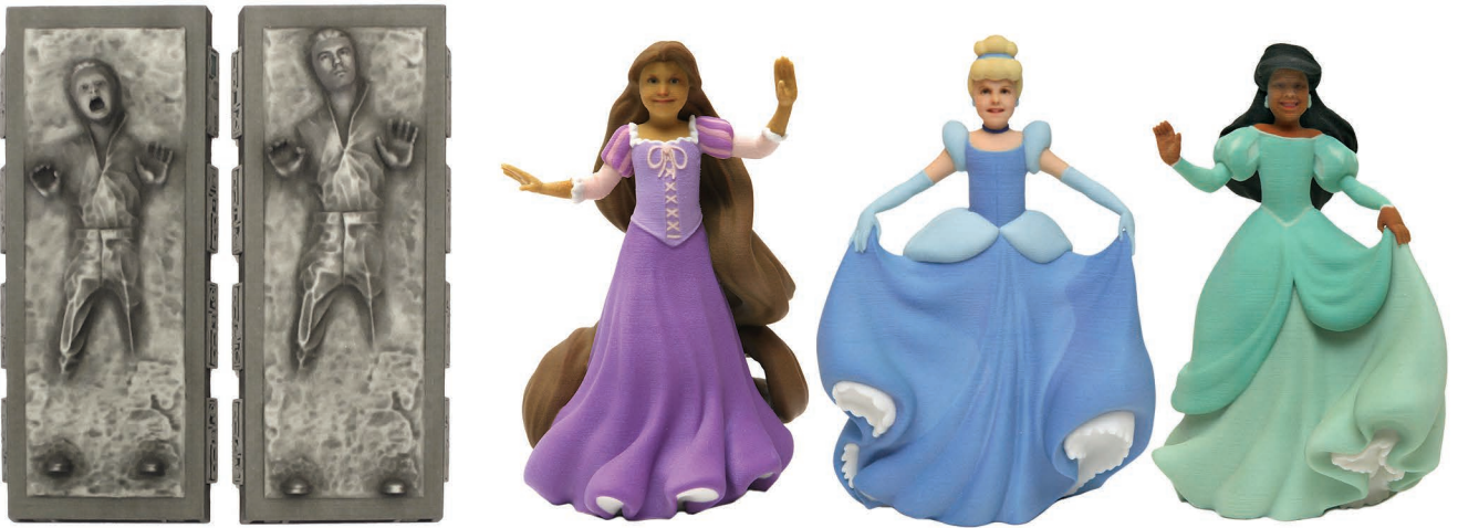
Figure 1. Figurines fabricated by our system. The system seamlessly integrates 3D facial data with a predefined figurine body into a unique, continuous object that's fabricated as a single piece by 3D printing.
