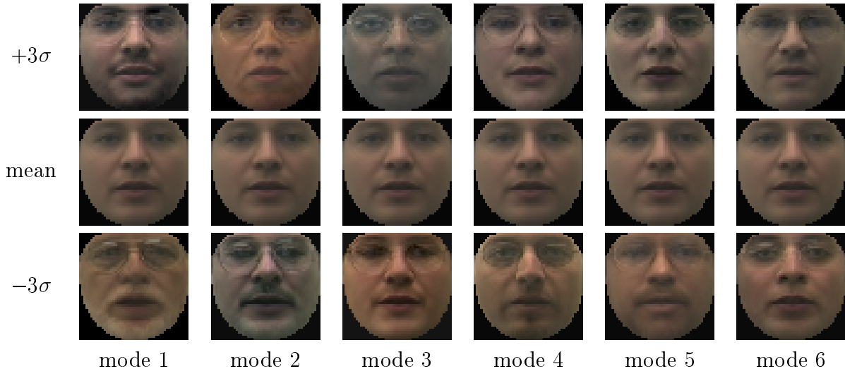
Figure 3.6: Shape free appearance. Center row: Mean appearance. Top row: Mean appearance +3 standard deviations ( +3\sigma ). Bottom row: Mean appearance -3 standard deviations ( -3\sigma ). The top six modes describe 41% of the training set variance.
