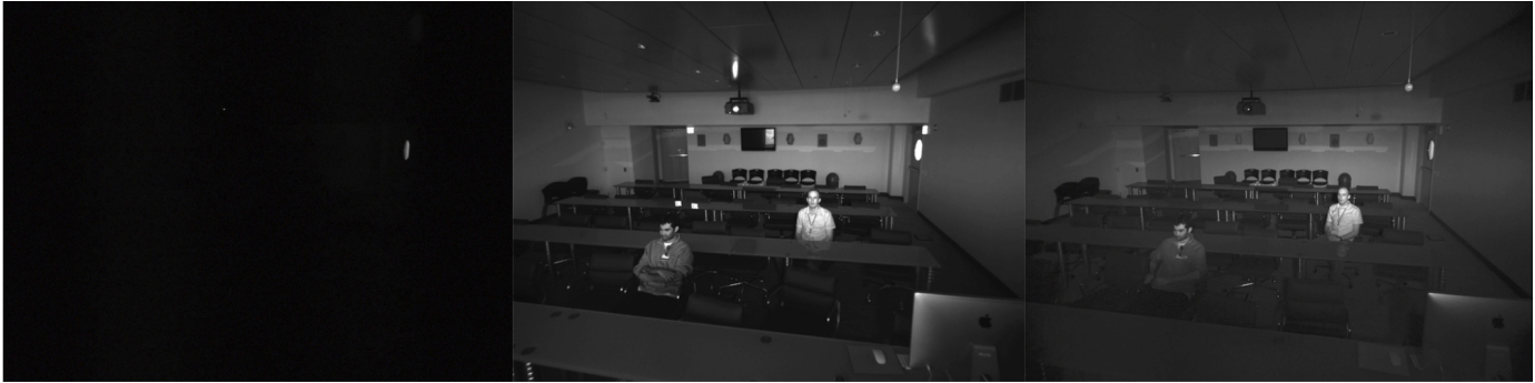
Fig. 2. (Left) Capturing video in a movie environment without IR illumination. (Middle) Example of the screening room with IR illuminators on – reflectance from the screen is problematic. (Right) We used an IR band-pass filter to remove the illumination reflected from the screen to obtain a uniform lighting environment.
