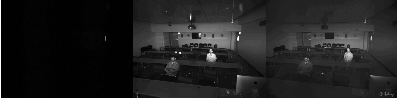
Figure 3. (Left) Capturing video in a movie environment without IR illumination. (Middle) Example of the screening room with IR illuminators on - reflectance from the screen is problematic. (Right) To remove the reflected illumination from the screen we used a band-pass filter to obtain a uniform lighting environment.
