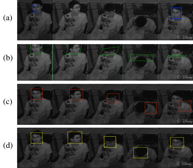
Figure 7. Examples of various face detectors/trackers: (a) Fraunhofer face detector fails due to the low light conditions, viewpoint (camera is looking down on the audience) and resolution of the faces are small (b) Template tracking method fails when there is pose/appearance change, (c) l_1 tracker breaks when the key frames are not in the dictionary, and (d) Modified l_1 tracker works reasonably well but requires key frames to be found manually.
