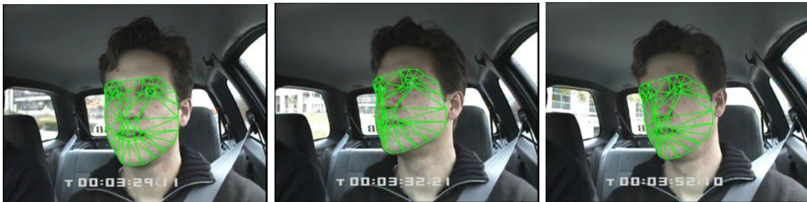
Figure 3: Example driver head tracking results with an AAM. View in color for the best clarity.
