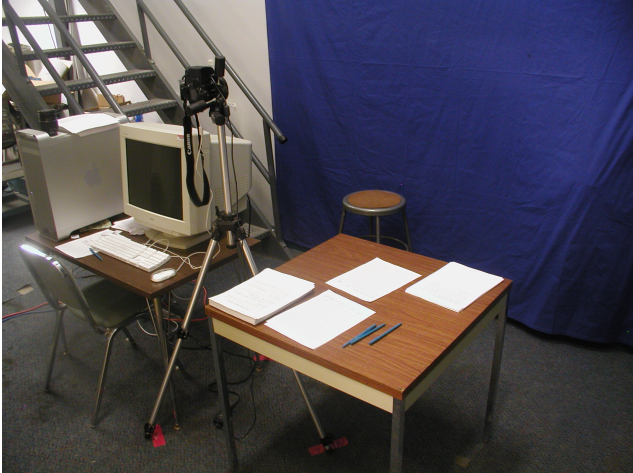
Figure 2. Setup for the high resolution image capture. Subjects were seated in front of a blue background and recorded using a Canon EOS 10D camera along with a Macro Ring Lite MR-14EX ring flash.
