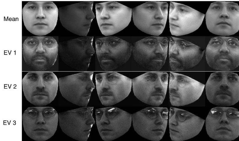
Fig. 8. The mean vector and the first three eigen light-field vectors for six poses of the PIE database. To best illustrate the eigenvectors, we display the mean vector plus a multiple of each eigenvector. That way, the eigenvectors actually look like real faces and are typical of the appearance variation in the eigenspace.
