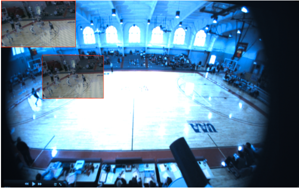
Figure 3: When the user switches to the iso-camera, the view is displayed in a highlighted red box and is also shown in the upper left corner of the interface to avoid occlusion from the user’s hand.
