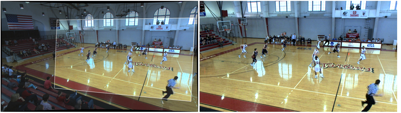
Figure 10: Spherical Resampling. The image captured by the robotic camera (left) at pan \phi_{\text{robotic}}(t - M) is resampled to synthesize the image of the virtual camera (right) oriented at \hat{\phi}_{\text{virtual}}(t) . Here, the virtual camera is looking further to the right than where the robotic camera had looked, which is why only pixels from the right side of the image are used for resampling.
