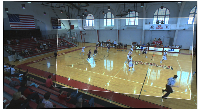
Figure 1: Hybrid Camera. We first use a robotic pan-tilt-zoom camera to follow the centroid of player positions estimated by a realtime person detector. After a short delay, we then resample the image to generate the video frame of a virtual camera (highlighted) which has a smooth camera motion trajectory because the path planning algorithm can take into account how the players will move in the immediate future (see accompanying video for full effect).
