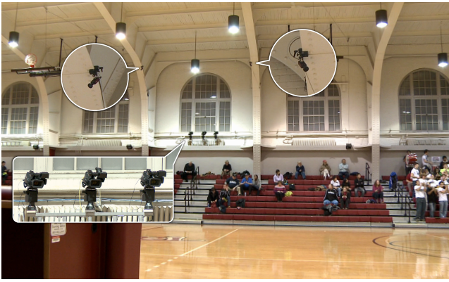
Figure 3: Experimental Setup. Two Allied Vision GX 1920C machine vision cameras mounted near the ceiling of the gym are used to detect and track the basketball players (see Fig. 4). Three Sony EX3 cameras situated behind the spectator seating at center court capture the broadcast video. Each camera is mounted on a FLIR D48-E robotic pan-tilt head. The motion of each camera is determined from either a human operated joystick, or an autonomically generated plan based on the realtime analysis of the player positions (see Fig. 5).
