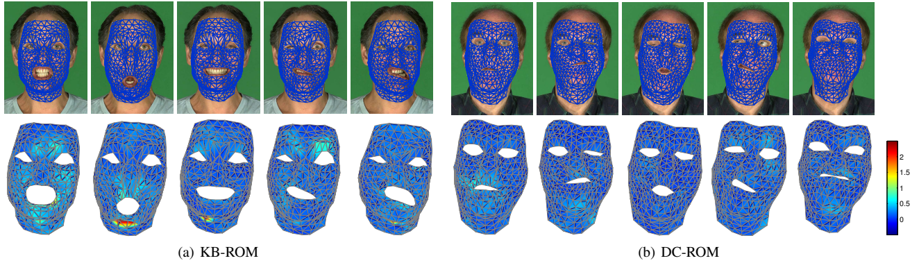
Fig. 9. Labeling results of Bilinear-DCT based EM algorithm. Sub-figures (a) and (b) show our labeling results projected on images (first row) and Bilinear-DCT reconstruction (second row). Colors indicate error in reconstruction with respect to the ground truth. Results show that Bilinear-DCT EM algorithm achieves similar accuracy as labeling by a professional, while significantly reducing manual effort.
